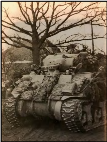
BCR Tank near Veen March, 1945 (Swift & Strong) This Sherman tank displays the changes over the year following the landings in Normandy with improvised armour in the form of tank tracks added to the hulls and turrets of the Sherman tanks.
